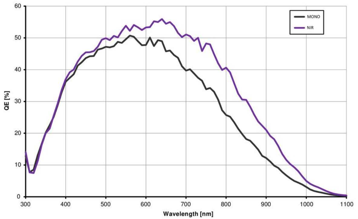
Image B-2: quantum efficiency curve for standard and NIR monochrome
